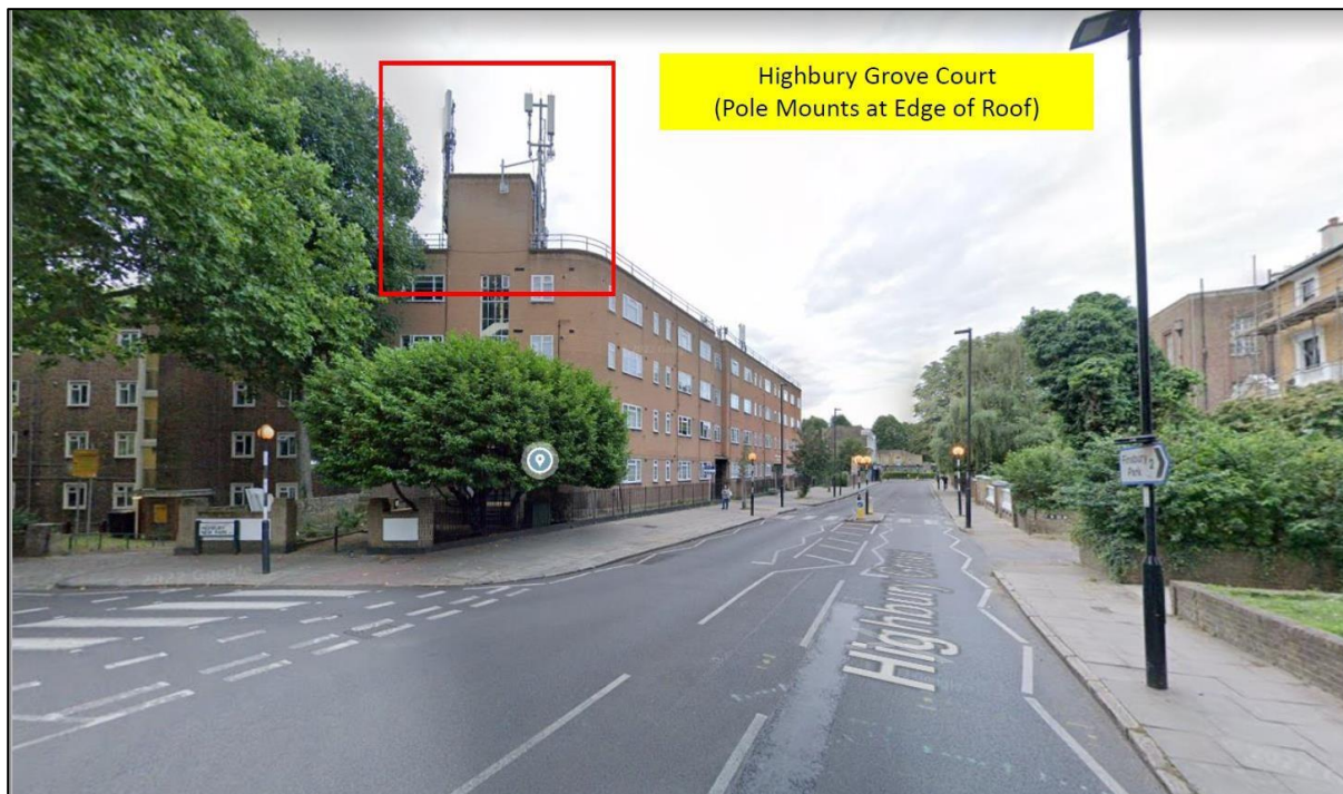
Image 4 - Examples of Pole Mounts on Highbury Grove Court (Not to scale and only for reference).
